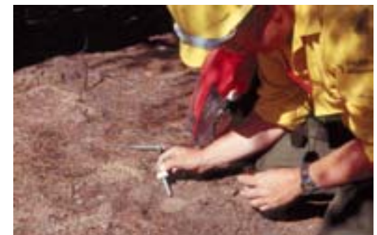
A simple test can determine whether a water repellent layer is present.
